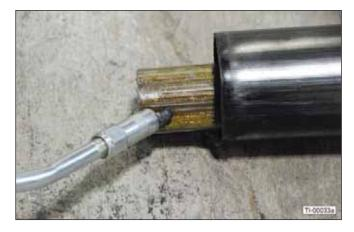
20. Slide the front driveline half over the rear half. Align the square rib on the mating halves to engage.
