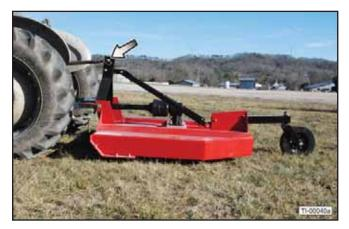
4. Disconnect the lift arms and remove the rotary cutter driveline from the tractor PTO shaft. Lay the driveline down carefully to avoid damaging the driveline or its shield. Do not let the driveline fall into mud or dirt, which can contaminate the bearing and shorten the life of the driveline.
