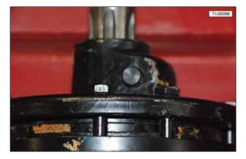
19. Apply a bead of grease around the end of the inner drive shaft.
