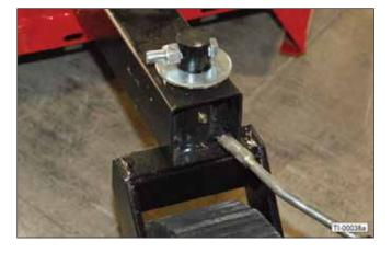
25. Apply grease to the zerk on the tailwheel hub.
