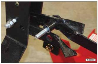
5. Tighten the bolt sufficiently to eliminate side play, but still allow the break link to function.
