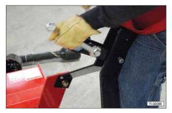
4. Position the back braces on the outside of the break link and reinstall the bolt. Be sure the spacer is in place.
