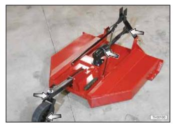
Grease all zerks every fifty hours of operation. Use an SAE multipurpose high-temperature grease with extreme pressure (EP) performance. Also acceptable is an SAE multipurpose lithium base grease.
