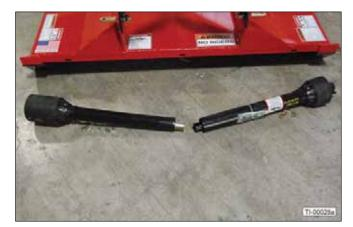
10. Depress the tab on the implement end of the driveline and slide the outer shield down and away from the U-joint.
