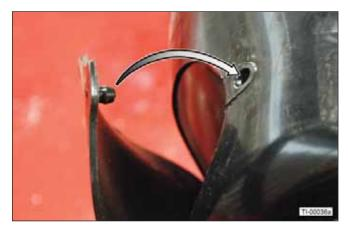
23. Attach the chain on the outer shield to the rotary cutter.
