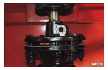
18. Install the retaining bolt and tighten the locknut.
