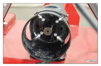
15. Separate the two halves of the driveline.
