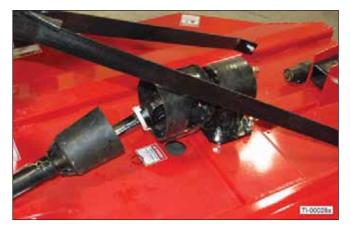
12. Install 1/2-13 x 3" Grade 2 shear bolt (11) and lock nut (12). Install the snap ring in the groove on the input shaft (shown by arrow).
