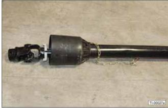
11. Slide the driveline onto the gearbox input shaft. Align the shear bolt holes in the shaft and the U-joint.
