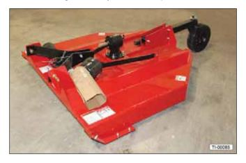
2. Cut the wires holding the driveline parts to the A-frame. Set the driveline aside for now.
